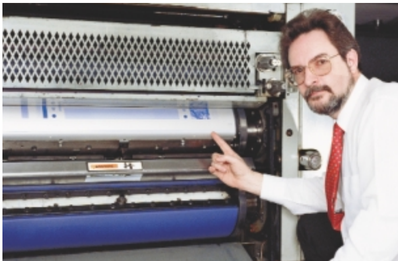
A thin scum line on the plate bend indicates good ink/water balance.
